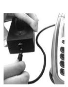
Then connect the other cable to the power supply unit and connect the twin pronged electrical plug to an electrical point
